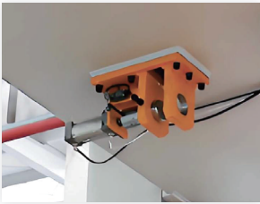
upper limit safety cylinder of slider
