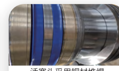
活塞头采用铜材堆焊 The piston head is surfacing welded with copper
