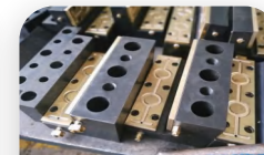
加强高精度滑块导向结构 Enhanced high-precision slider guide structure
